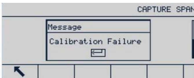
Figure 1-19: Span Calibration (Failed)
