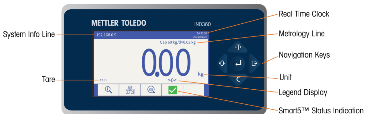
Figure 1-12: IND360 Panel Mount Front Panel Layout
