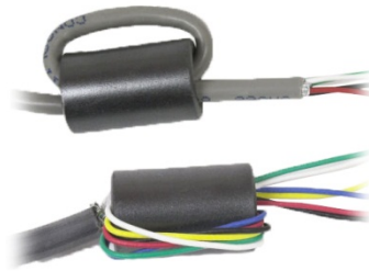
Figure A-24: Installing the Ferrite Cores
