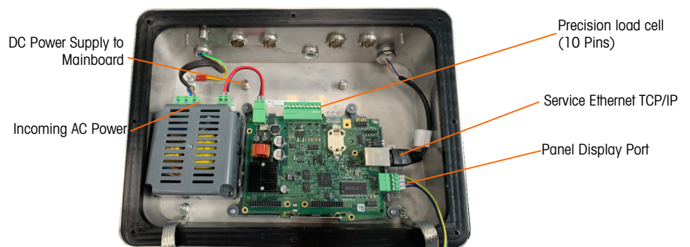
Figure A-36: Precision Main Board in Harsh Enclosure
