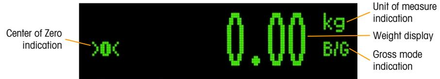
**Figure 2-1: Display in Weighing Mode**
