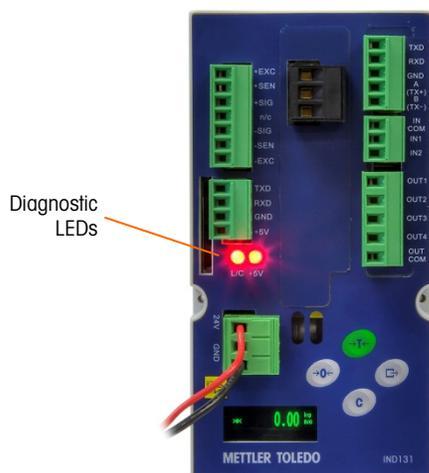
**Figure 4-1: Diagnostic LEDs**
