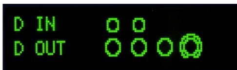
**Figure 3-19: Discrete I/O Test Display, Output Active (bottom)**
