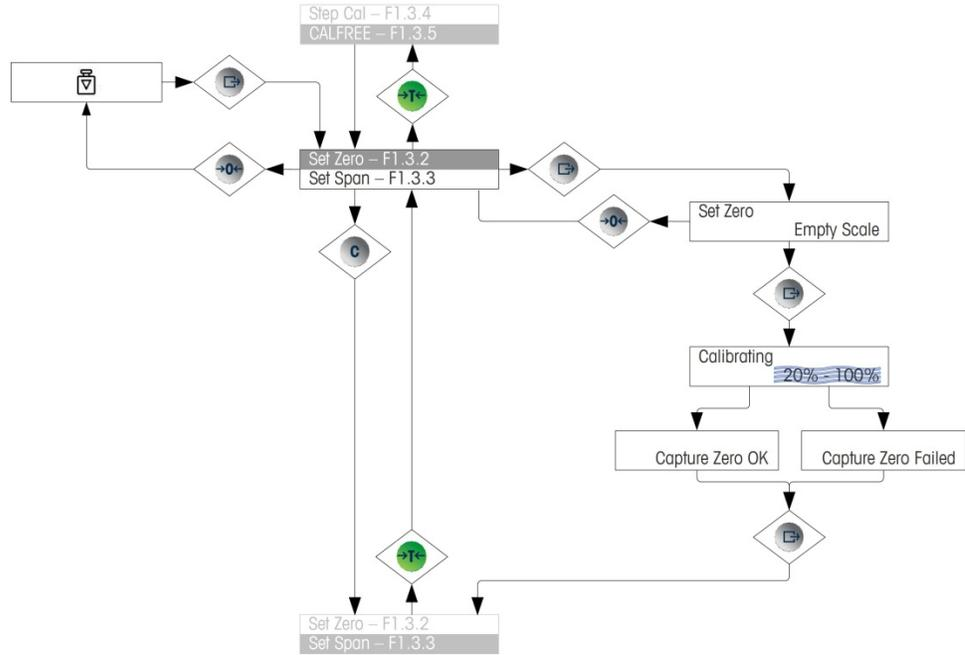
**Figure 2-11: Zero Calibration**
