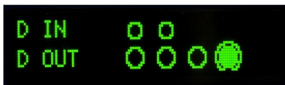
**Figure 4-6: Discrete I/O Test Screen, One Output Active**
