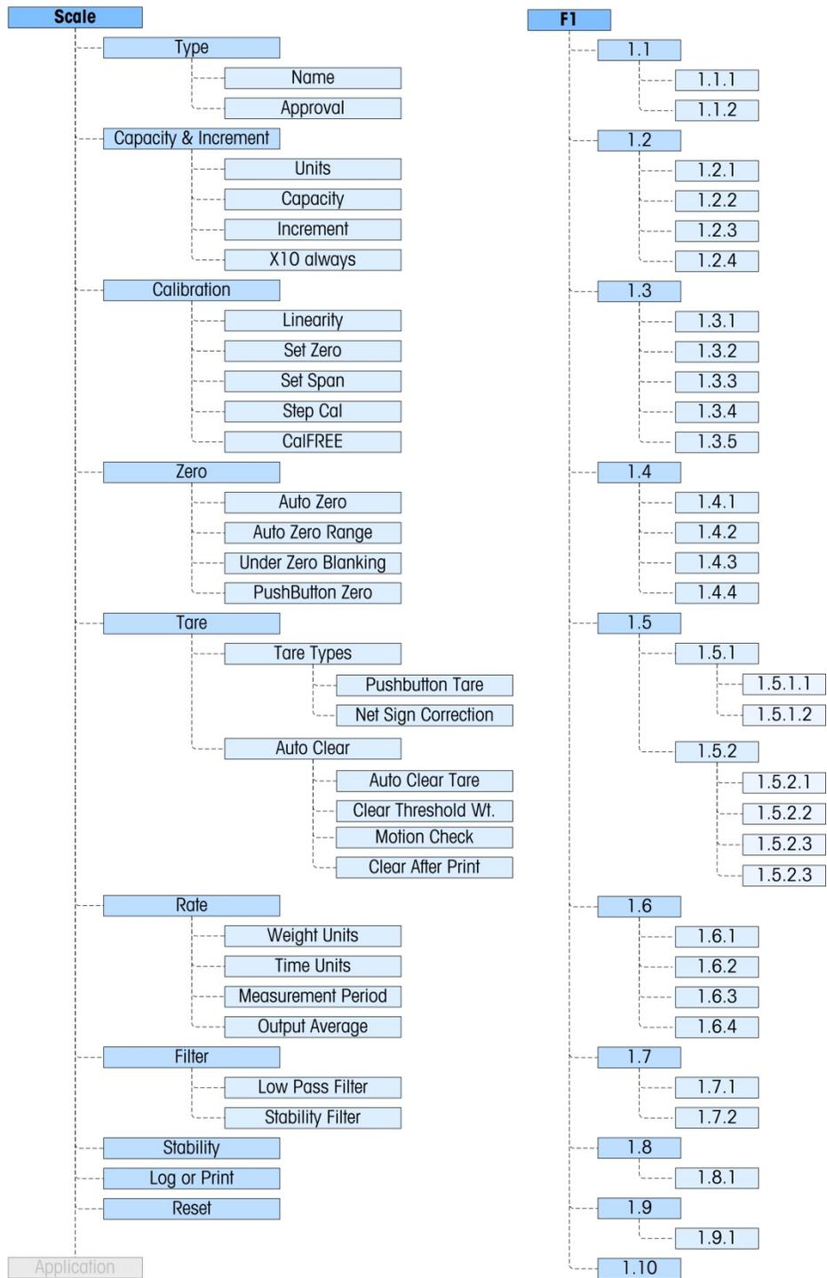
Figure 3-6: Scale Branch of Setup
