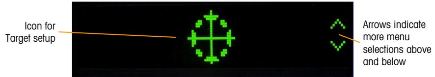
**Figure 2-2: Display in Operator Entry Mode, Target Icon Displayed**
