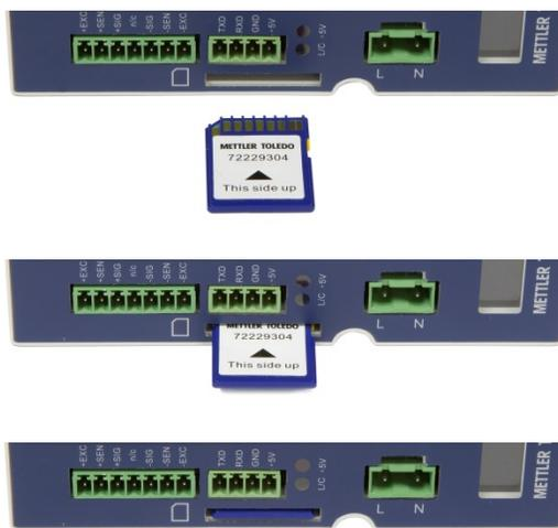
Figure 4-7: SD Memory Card Insertion, DIN Terminal
