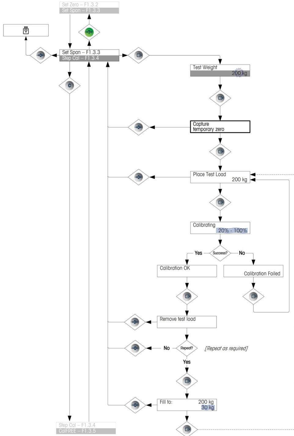
Figure 2-13: Step Calibration
