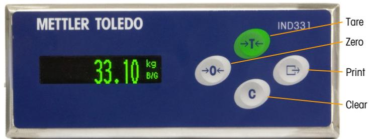
**Figure 2-3: IND131/IND331 Scale Function Keys**
