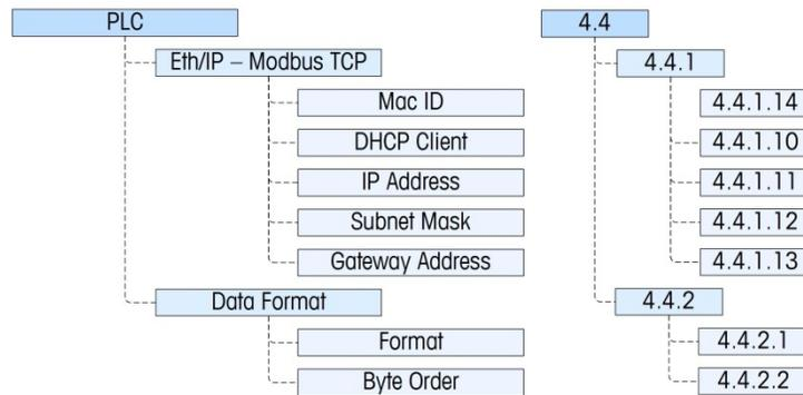
**Figure 3-15: Setup Menu for Ethernet/IP and Modbus TCP**
