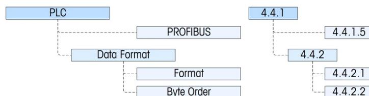
**Figure 3-16: Setup Menu for PROFIBUS**
