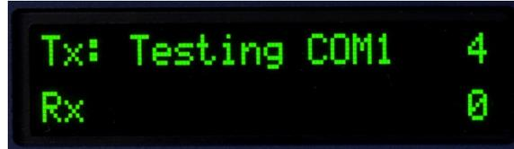
**Figure 4-3: Serial Test Display**
