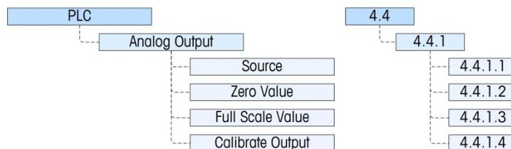
**Figure 3-10: Setup Menu for Analog Output**
