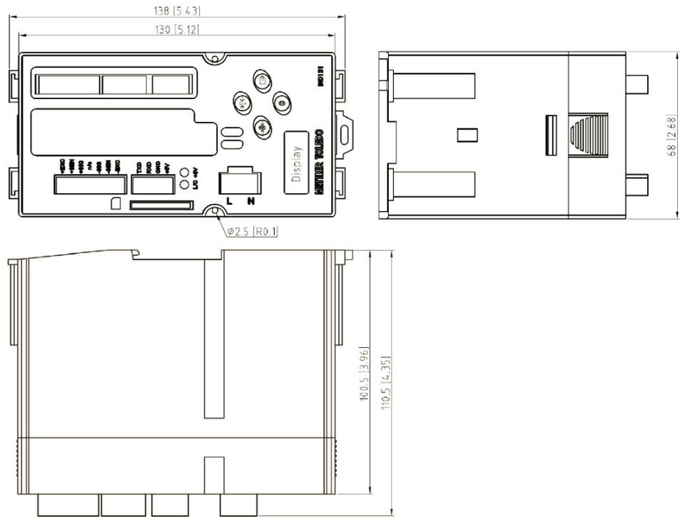
Figure 1-2: IND131 DIN Rail Mount Enclosure Dimensions
