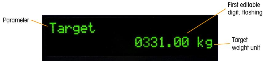
**Figure 2-7: Target Entry Screen, Value in Focus**
