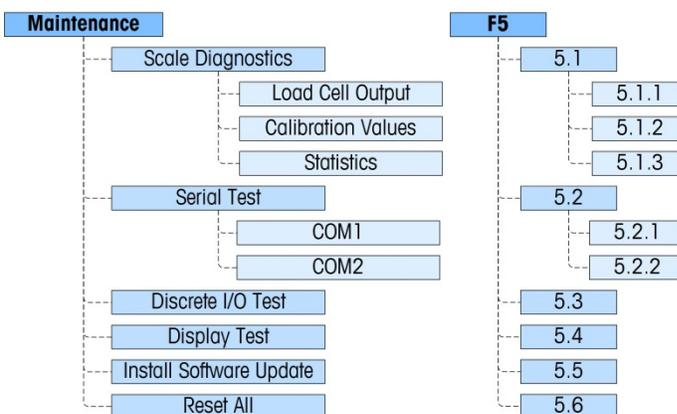
Figure 3-17: Maintenance Branch of Setup
