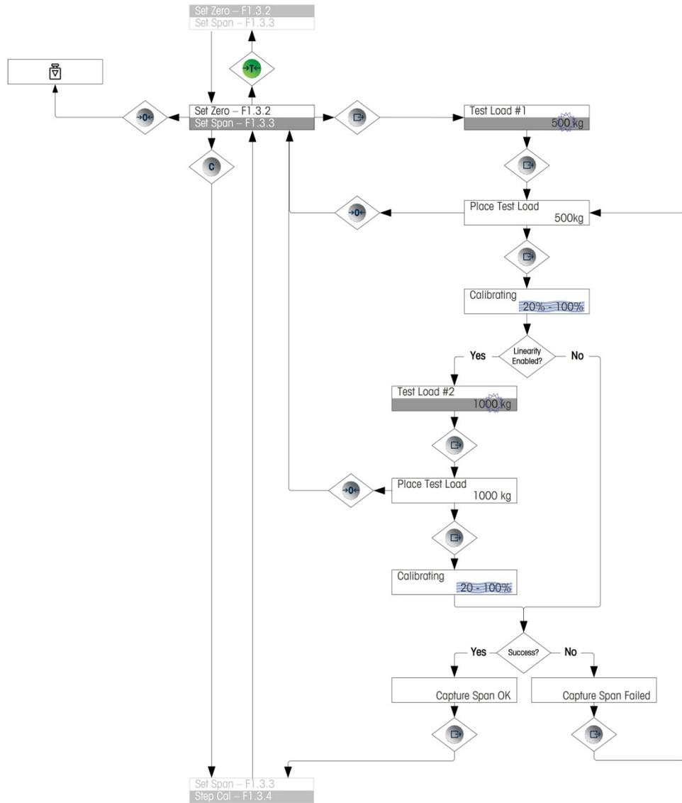
Figure 2-12: Span Calibration
