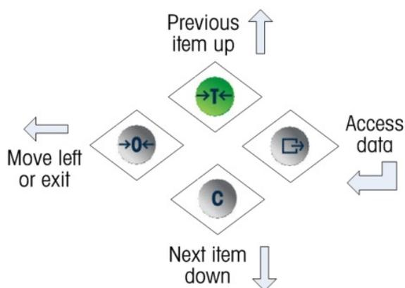
**Figure 2-4: Key Functions When Viewing the Operator Menu**
