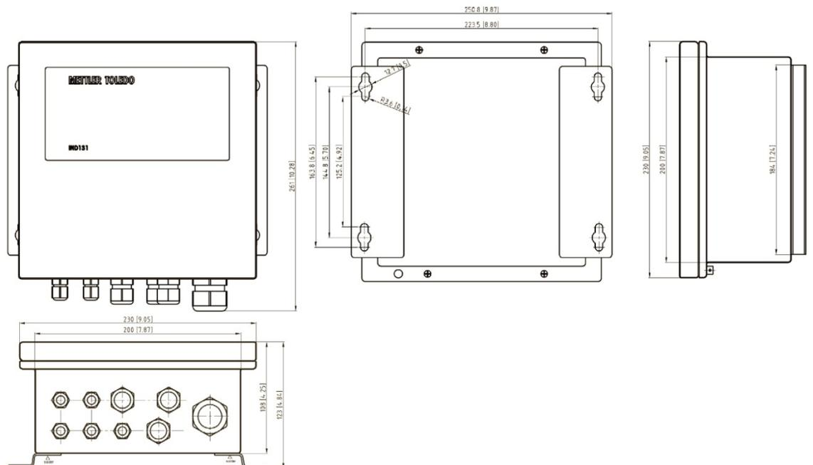
**Figure 1-5: Original IND131 Junction Box Enclosure Dimensions**
