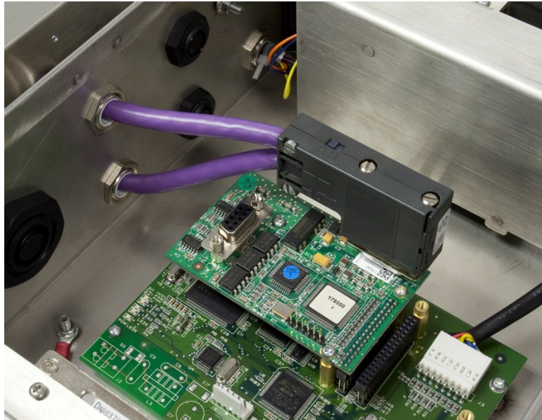
Figure 3-22: PROFIBUS Connection in ACM500
