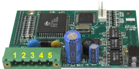
Figure 3-25: DeviceNet Option Board
