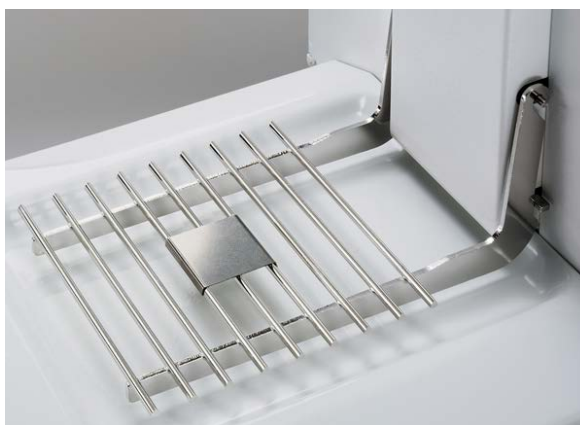
Figure 3-3: Weighing pan designed as a grid Grids can help to reduce the influence of the air draft, especially for 5th and 6th decimal points
